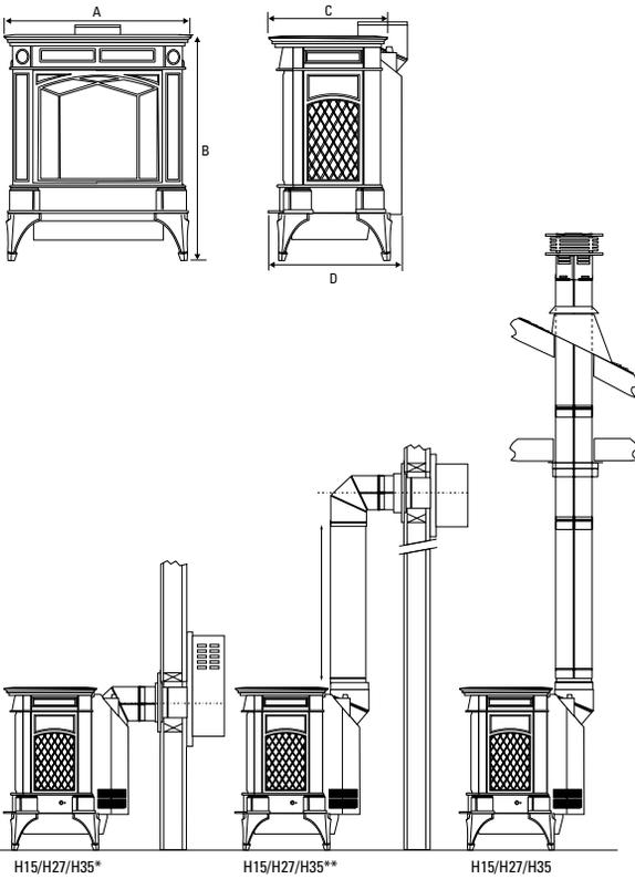
\* The H15 can be vented horizontally with the AstroCap™ system. For rear vent applications, H27 requires a riser vent; H35 requires a riser vent and BTU reduction kit.
